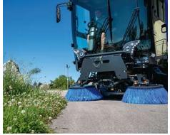
A flexible sweeping system helps ensure thorough cleaning in any situation. The towed disc brush system, mounted in front of the front axle, achieves a sweeping width of 86.6 in.
