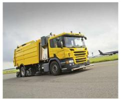
Additional spray bars convert the Schmidt AS 990 into a stand cleaning machine (ASC 990).
