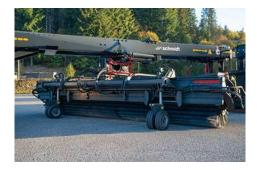
The twin castors offer very quiet, vibration-free and smooth sweeping performance, while level snow ejection and the cleanest fine clearing ensure maximum safety. This is achieved thanks to aerodynamic spoiler guidance, automatic spoiler adjustment and wear-dependent brush speed adjustment. This permits the jet sweeper to deliver a specific fine clearing result, while the robust design offers both optimum operational capability and maximum safety.
