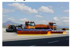
Clean and aggressive clearance is achieved with the Schmidt MS Tarron airport snow ploughs, such as the MS 56.2 NA. These are designed for fast snow clearance at airports and offer outstanding performance with optional fine clearing bar, ejection stop or low blade shape.
