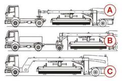
With different coupling systems, we offer a wide selection of jet sweepers that are perfectly tailored to your individual requirements. By using a modular system that includes various TJS versions, working widths and clearing capacities, a customised TJS/TJS-C can be configured to meet your exact requirements. Within the coupling systems, we distinguish between three different variants:
