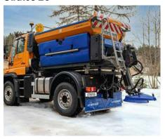
The eStratos 25 is a silo spreader with a hopper capacity of 2.5 m<sup>3</sup>.
