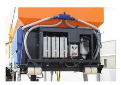
the eStratos is significantly quieter. In addition, the safe 48 V DC system can be maintained without special training or safety measures.
